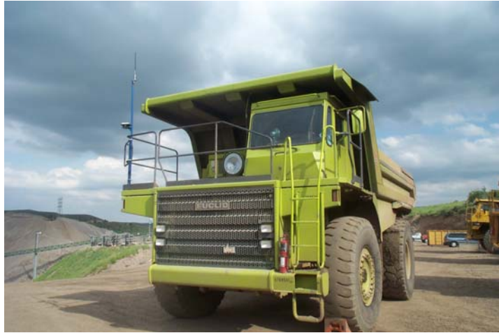
Figure 7.1: Mounted GPS and Wireless Antennas on a Truck [55]
