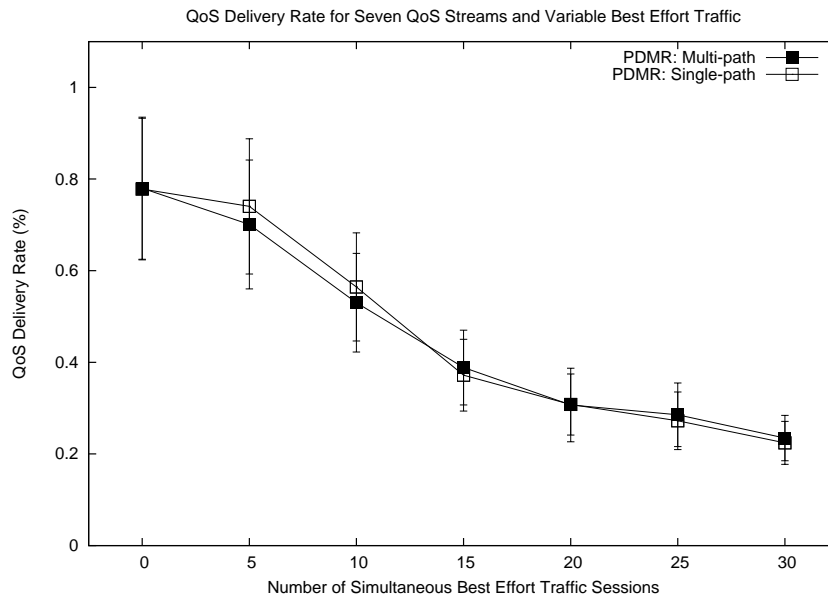
FIG. 5.13. QoS delivery rate for a mobile network with seven concurrent QoS traffic sessions as the number of simultaneous best effort traffic sessions varies
